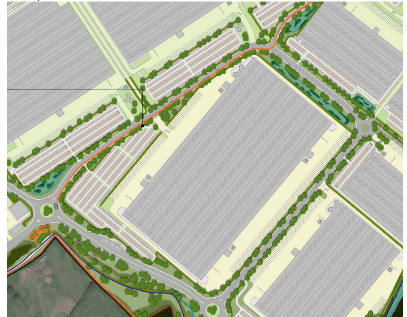
Fig 16. Internal Distributor Road, extract from illustrative landscape strategy plan, illustrating the notional alignment (in orange) of the dedicated Public Right of Way within the main site, and connection options to the new bridleway and existing Public Right of Way
