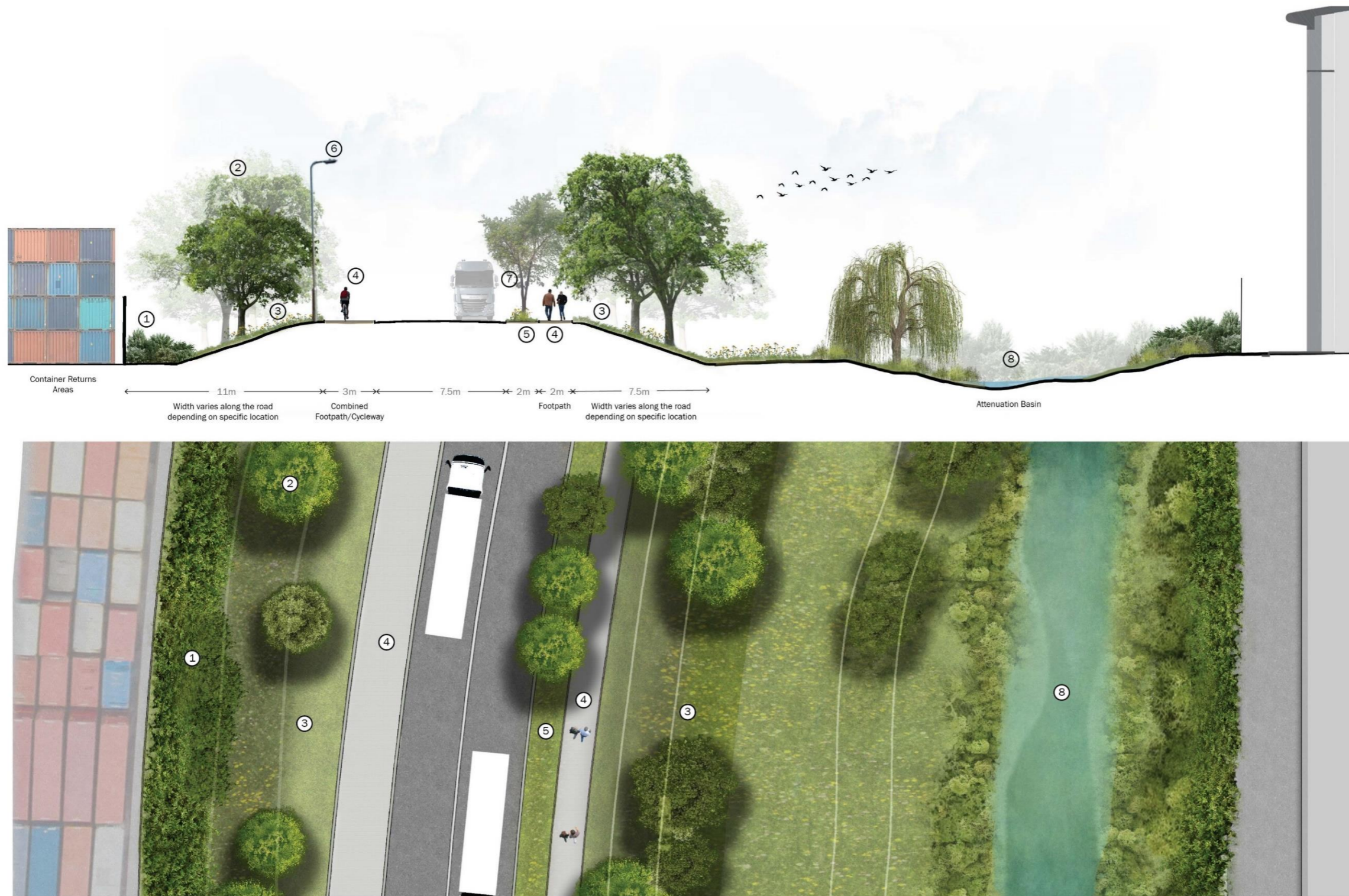
Fig 15. Typical Sections through A47 Link road (2 of 2) – Numbers relate to Design Code Text below
